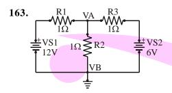
Find the node voltage  $V_{\Delta}$ .
