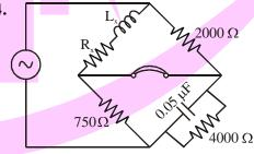
In the Maxwell bridge as shown in the figure the values of resistance  $R_x$  and inductance  $L_x$  of a coil are to be calculated values are shown in the figure at balance. The values of  $R_x$  and  $L_x$  will respectively be
