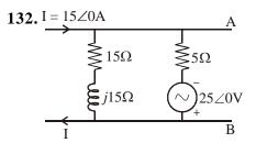
For the circuit shown, the Norton's equivalent current source as terminals A & B is given
